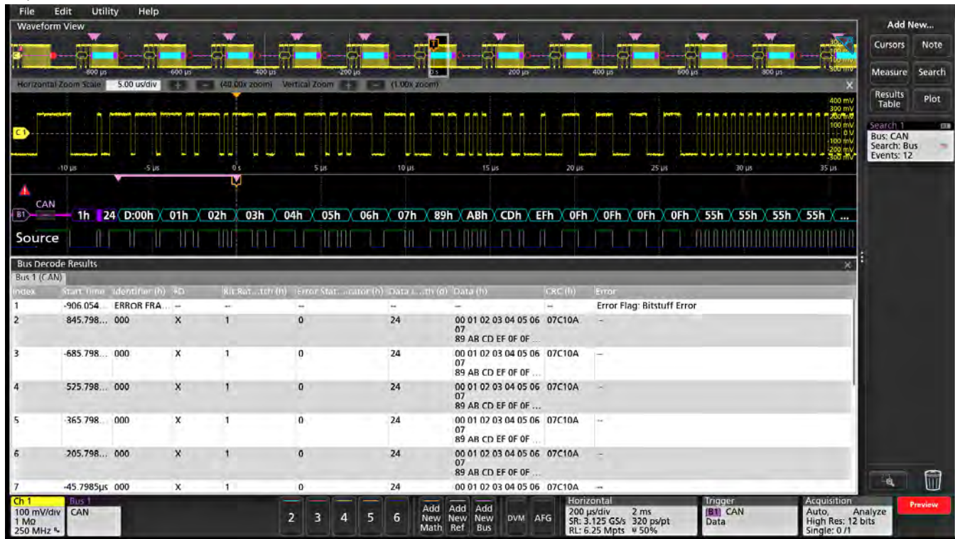
Figure 23: Triggering on a CAN serial bus. A bus waveform provides time-correlated decoded packet content including Start, Arbitration, Control, Data, CRC and ACK while the bus decode table presents all packet content from the entire acquisition.
