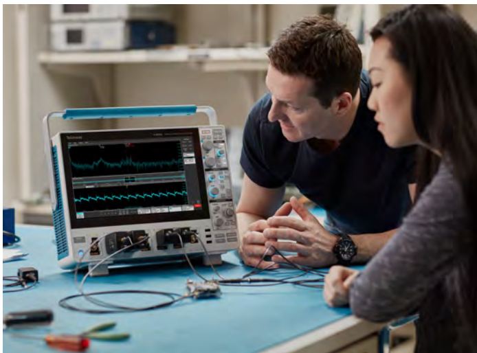
Figure 1: Voltage measurements on a switch-mode power supply showing the ripple voltage on one of the power rails.
