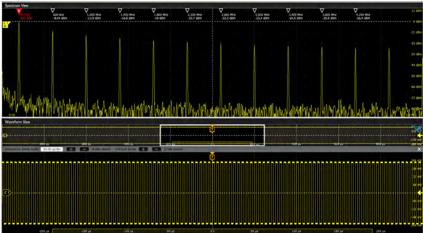
Figure 25: Spectrum Time gates the range of time where the FFT is being calculated. Represented by a small graphical rectangle in the time domain view, it can be positioned to provide time correlation with the time domain waveform. Perfect for conducting Mixed Domain Analysis. Up to 11 automated peak markers provide frequency and magnitude values of each peak. The Reference marker is always the highest peak shown and is indicated in red.
