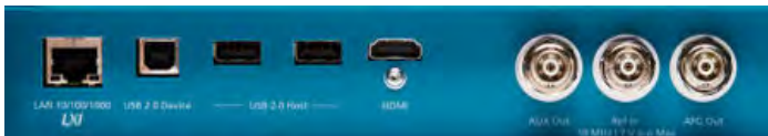
Figure 30: The I/O you need to connect the 4 Series MSO to the rest of your design environment.
